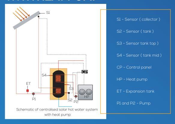
The diagram explains how solar collectors and heat pumps work together and heat up the water in the storage tanks. The storage tank shown in the diagram is a twin coil for the solar heating source and secondary heating source (in this case heat pump). The system has an automated control system to switch on and off of the heat pump(s), depending on the heat load of the building.
